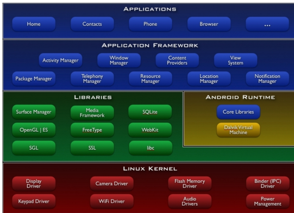
Figure 2.2: The Components of the Android Operating System
